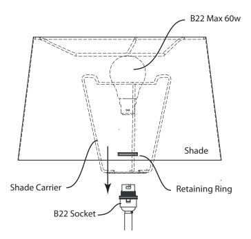
For your convenience your floor lamp comes fully assembled. Please take care when moving the lamp to not damage or put unnecessary force on the flexible cord.
